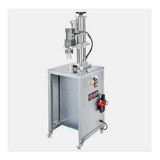
The container cap closing equipment is semi-automatic capper. It is suitable for object container with plastic screw caps.
