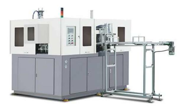
Hand feeding Jar making machine is a type of machine between semi-automatic and fully automatic machines. Only need worker to feed preform, the machine action of blowing and bottle dropping are fully automatic. Suitbale for the neck from 38mm to 120mm.
