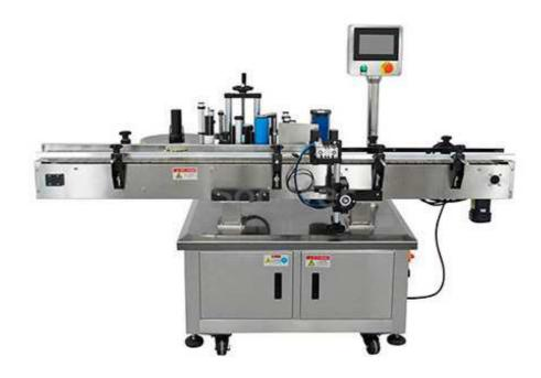
This is a high-speed round bottle labeling machine, which can quickly apply labels to wine bottles, water bottles and other round bottles.
