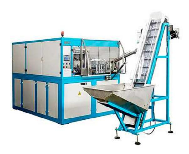
Master Packing manufacturing design and produce the fully automatic bottle blowing machine more than 20 years, now we can produce 1-16 cavity, 10ml-30L PET blow bottle machine with the output 100-19200BPH. All Master blowing bottle machines can connect to the filling line. Master packing supply pet bottle blowing machine mold and preform and cap injection mold. Our quick change blow mold can save a lot of time and effort on change mold.
