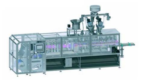
Our firm's last product, DPM60 doypack Machine, is presented to stretchy packaging sector by our research-development engineers. It is a fast machine that makes filling through making package from bobbin. It can present wide range of packaging of liquid, powder, granule types of food and cleaning goods. Machine can present advantages in the innovative packaging. With the DPM60 Doypack Machine, it is possible to take product outputs with zipper and nozzle capped.
