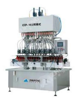
The machine is a high-tech filling equipment controlled by microcomputer PLC programmable as a whole. In order to achieve high filling speed through add times filling heads, doule line and filling alternately. Features are as follows: high production speed, accurate measure, no drop and no foam appearance. This product mainly use for packing all kinds of bottle and suit for water aqua such as foodstuff, cosmetic, daily chemical, pesticide and fine chemical products.
