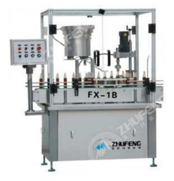
The machine can automatically operate a whole process of bottle sending, bottle cap unscrambling and cap covering. After dial positioning, single-head manipulator is used for cap grasping and cap screwing. With simple operation and easy maintenance, this machine is applicable for the capping and sealing of various cap-screwed bottles.
