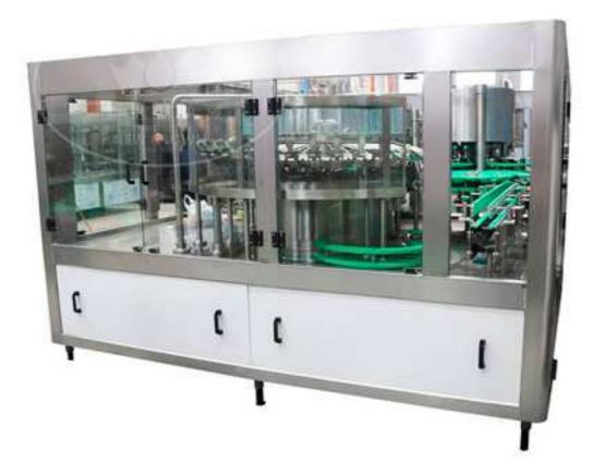
Our newly designed CGF serious monoblack water filling machine is designed for plastic bottle filling, it can suit for PET bottle size between 150ml to 2000ml, can customized to maximum of 3000ml. Genus design of capping design makes different screw cap change into one simple easy torch. On machine surface is only leaving 3 points of bearing support point which makes drainage so easy and without any dirt stain.
