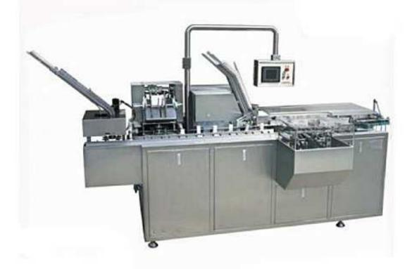
SPJ100 Fully Automatic Cartoning Machine applies to the encase packing of blisters, vials, cosmetics and similar stuff. This machine can fold leaflet, open carton and insert stuff with leaflet into cartons, printing batch number and close carton automatically. This machine adopts horizontal configuration, PLC control system, photocell detector installed in each station enables stable running.
