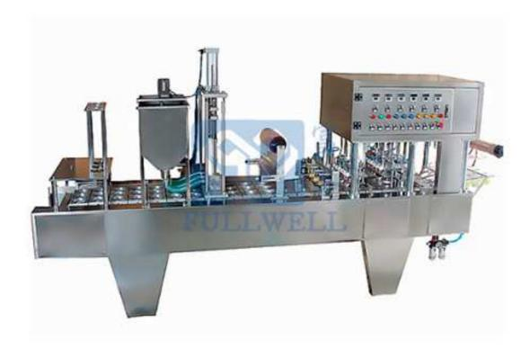
This cup filling and sealing machine is a multifunctional high-speed fully automatic machine specially designed for liquid or semi-liquid (such as water, milk, yogurt, olive oil, fruit juice, tomato sauce, honey) to be filled and sealed. The machine applied with world famous electrical and pneumatic components. High quality, high stability, long service life. All the parts of this cups filling and sealing machines are made of food grade #304 stainless steel.
