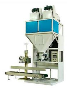
Semi auto rice filling sealing machine can suit for different type bags such as woven bags, Kraft bags, paper bags etc, and bag closed by sewing/thread stitching or heat sealing/hot sealing.
