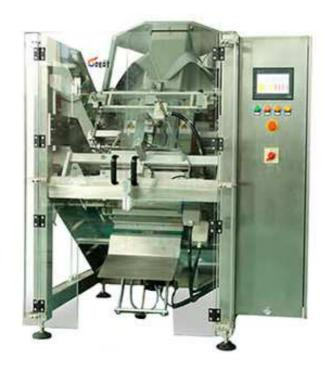
Inclined Type VFFS Packing Machine GP800, suitable for Fragile product heavy pouch packaging, such as biscuits, jelly, etc. The frame of the machine has enough rigidity, which is durable&Long service lifetime. Reasonable structure and each lane separated control also User frinedly& easy for maintenance. It also set up the safety door to protect user safety.
