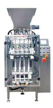
This is a fully automatic multi-lane stick bag machine for packing sugar or coffee. The machine is able to dose the required grams, make the stick bag or side bag, then fill the sugar or coffee into the bag, seal, and cut. Lot number printer is optional.
