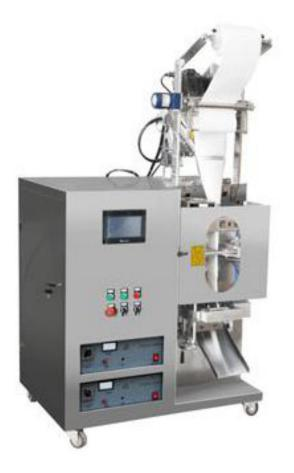
The MK-388FM vertical form fill seal machine is designed to perform automatic film pulling, bag forming, filling, weighing, sealing, cutting, counting, heat printing, and finished package conveying. Non-woven fabrics are used to make packaging bags and an ultrasonic sound is used for sealing, offering aesthetically pleasing packages. With the auger filler, this packaging machine is suited to package -100 mesh powdered products like lime powder, foot bath powder, and more.
