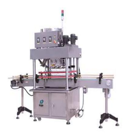
The press and capping machine PAC-1P is used to press caps and screw caps after filling machine. It is suitable for most kinds of screw caps. Widely used for cosmetics/medical/chemical/food industry. And it can be linked with filling machine and labeling machine in line.
