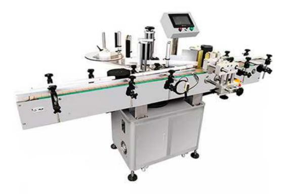
Achieve automatic labeling the adhesive label on round surface or small conical surface of the products.
