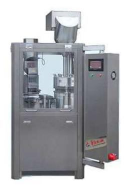
It adopts multi-bore dosing, batch-type rotating and speed frequency controlling. It includes whole capsule filling process: capsule sowing, separating, filling, un-separated capsule rejecting, closing, and filled capsule outputting. The machine is suitable for filling both powder and pellet.
