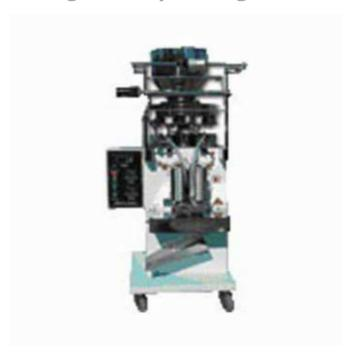
The machine is used to fill and seal more granulates automatic, and sachet sealing shape is four sealing shape, It can be used to package beans seed medicine salt drying agent spice tea etc. The advantage of the machine is measure device adopting unloading door turning and returning new techniques, high speed and little noise.
