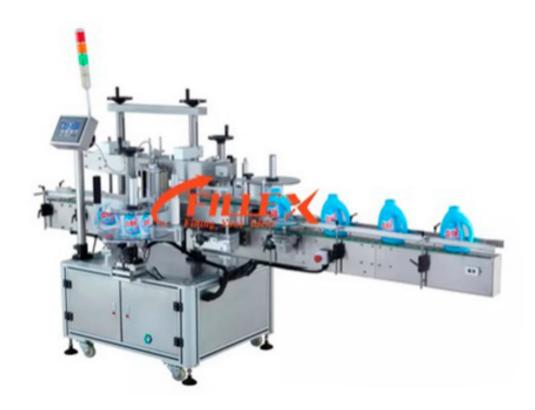
This equipment is suitable for gluing and labeling of various round bottle objects. Paper separation, gluing, labeling and labeling are automatically completed, reducing manual labeling procedures and improving labeling efficiency. Glue is evenly applied, with filamentous stripes, no wrinkles, and improves packaging quality. Especially suitable for small and medium batch labeling production, such as labeling of food and wine.
