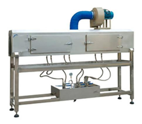
The steam label shrinking tunnel is widely used in food and beverage industry, Chemical industry, pharmaceuticals industry etc.
