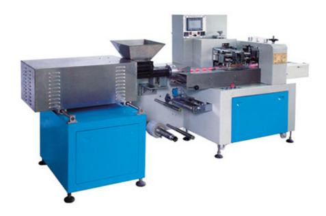
This machine is suitable to pack color plasticize clay automatic packaging, can be done automatically plasticize molding cutting and packing and automatic print date has a high degree of automation, packaging, speed and stability characteristics, servo system control small foodprint, simple open ration, easy to use.
