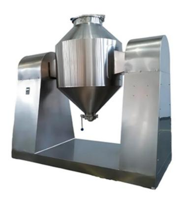
The Machine is a multi-functional high-efficiency mixing equipment has stable performance, good usability, and reliable quality, which has been approved by the authoritative third party. No centrifugal force, no gravity segregation, stratification, accumulation phenomenon, each component can be mixed evenly under the weight ratio of the hanging beads, the filling coefficient can reach more than 40%, not more than 60%.
