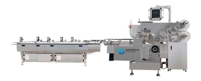
YB-DN260 model is specially designed for single twist/top twist packing style. Clever structural design, make the wrapping paper more fit, the kink is tight. By replacing the molds suites to achieve wrapping of multiple sizes of products.
