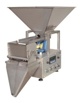
This is a machine that has been designed specifically for use in the packaging industry. It accurately measures and dispenses an array of products: granular, powdery, or small-piece items such as noodles. This equipment uses a linear weighing method in which products are evenly distributed over a linear conveyor belt system and then weighed individually before they are discharged into containers or packaging bags.
