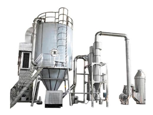
Basic Principle: High-speed centrifuge atomizing for the extract of traditional Chinese medicine is an application of centrifuge atomizing technique. It also uses high-speed atomizer to make liquid material into foggy droplet to contact with hot air fully to finish instant drying and get final powder product.
