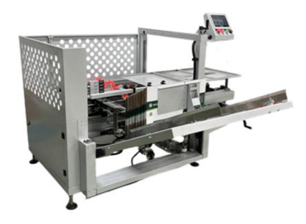
Carton Assembling Machine, are machines that automatically form cardboard boxes. These machines are commonly used in manufacturing and packaging facilities to improve efficiency and reduce human error. It come in different sizes and models, and can be customized to suit different applications.
