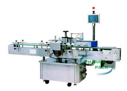
Bottles are fed into conveyor via bottle separator. A product sensor detects the presence of a bottle, instructs to dispense a label. Liner is reminded and the motion is controlled by a label sensor. Side conveyor enhances the labeling performance.
