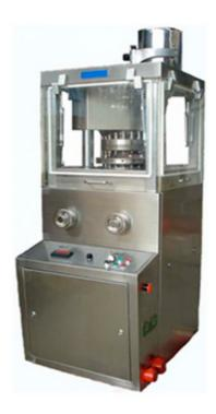
This machine is a single-press type, continuous automatic tablet press for pressing the granular raw material into the round tablets and irregular tablets etc. It is especially caters for small-batch production.
