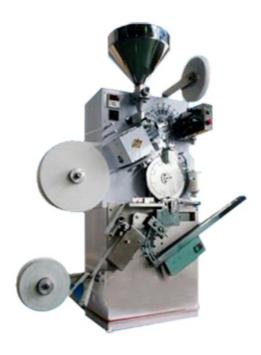
Tea bag packing machine Model CCFD6 features such functions as automatic ration filling, heat-sealing of tea bags, automatic plastering of cotton thread and tags, and cold-sealing of the envelope in the longitudinal direction.
