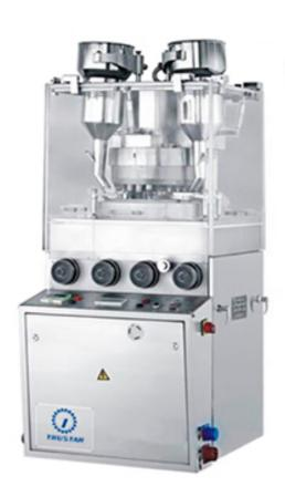
This model is to press the various kinds of granular materials into tablets, with the most outstanding advantage of being able to produce irregular tablets with wide different geometrical shapes, such as double layer tablets, ring shape tablets and double side engraved tablets.
