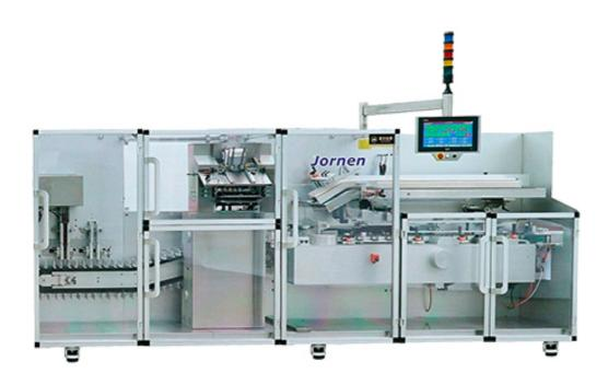
ZH400 is a Continuous Motion Cartoning Machine. It is suitable for pharmaceuticals, food, household chemicals, hardware, and electrical industries for the packaging of blisters, bottles, vials, pillow packs, toothpaste, etc. It can fold leaflets, open cartons, insert the products and leaflets into cartons, emboss, tuck-in, or hot-melt closures and automatically discharge cartons.
