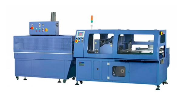
Auto Side Sealing Machine, standard model USA-005PR(CE) can adjust its packaging height basing on product to have strong seal & nice look.
