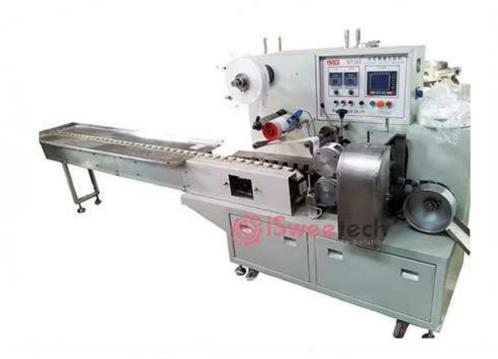
BP280 Flat-type Lollipop Wrapping Machine is suitable for packing flat lollipop sealed by two layers of films and is featured with superior, smooth and reliable performance. The packed candy is featured with good looking, good sealing, long period of storage etc. it is an ideal machine for packing all kinds of special shaped lollipop.
