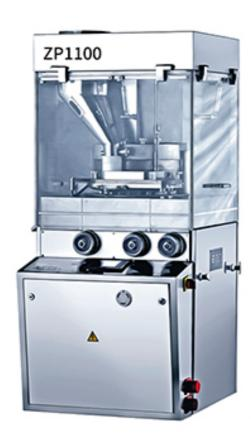
Model ZP1100 Series Rotary Tablet Press Machine is a new generation product. There is altogether four types. It is an economical high-speed tablet press machine and it is suitable for producing a great quantity tablets. It can be produced all types of round tablets, irregular tablets and tablets of engraved on double sides.
