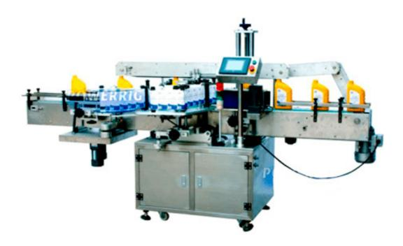
It is a side labeling machine, which is suitable for flat bottles, round bottles and square bottles with single-sided and double-sided labeling, such as flat bottles of shampoo, flat bottles of lubricating oil, round bottles of hand sanitizer, double-sided labeling, double-sided labeling, double-sided labeling, etc., which can improve the speed of production. It is widely used in daily chemical, cosmetic, petrochemical, pharmaceutical and other industries.
