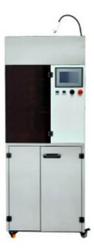
The Vacuum Decapsulator creates the air jet to transform 4-5bar compressed air provided by outside air source into the high-frequency pulsed vacuum. The high-frequency pulsed air continuously draws capsules in the working chamber within a certain period. As a result, capsules separate gradually; powder or pellets inside fall down into the barrel. Due to flexible forces instead of mechanical forces, capsule shells keep completely intact; no fragment created in this process
