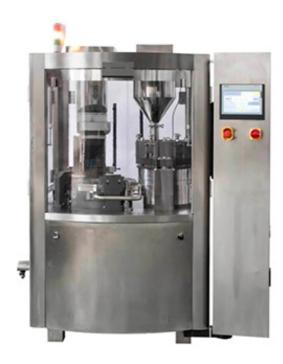
The fully automatic capsule filling machine is mechanical equipment for filling capsule drugs
