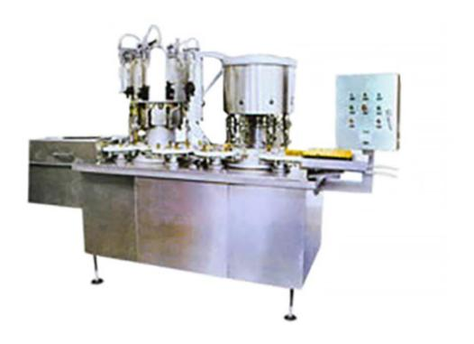
The SD-YGF-98 oral liquid filling sealing machine is a kind of filling close-over machine that is mainly used for the filling and closing-over productions oral-taken liquid, biology preparation liquid and so on. It adopts the vat-hanging circumrotating style, and can complete such procedures as the bottle-out automatically. This equipment can be used independently or connected with the completely auto-produce line.
