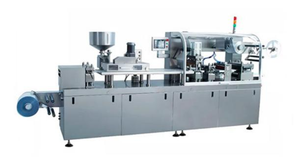
The machine is suitable for capsule, tablet, big honey pill, candy, liquid, paste, syringe, as well as irregular shape Alu-PVC, paper-plastic composite and Alu-Alu sealing packing in pharmacy, healthcare, food, cosmetics, medical equipment industry etc, fully comply with 'GMP'.
