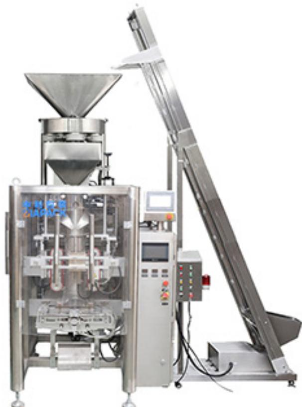
This unit machine is special design for packing various granule products like bean, rice, sugar, salt, grain and so on. Adopt the volumetric cup as dosing machine. Speed is fast and stable. The whole machine unit can reach the function of bag making, product weighing, filling, bag sealing and output. With date coding and bag counting which improve the automation. This machine is very popular in Modern small and middle factory.
