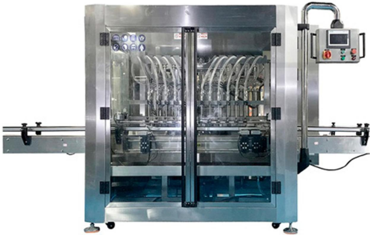
The automatic servo piston filling machine is a highly efficient and precise filling device widely used in industries such as food, pharmaceuticals, daily chemicals, and chemicals. It is capable of handling liquids, pastes, and high-viscosity materials. Its core advantage lies in its servo motor drive, which ensures high precision and flexibility during the filling process.
