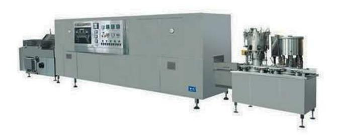
This oral liquid production line made in Shouda company is specially designed for the producing of 5-25ml oral taken fluid. It can finish all the process of ultrasonic washing, sterilizing, filling and capping completely by this line.
