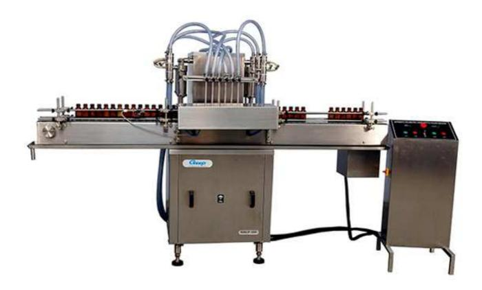
Automatic Volumetric Liquid Bottle Filling Machine work on volumetric principle with diving nozzles. The unit is made compact, versatile and enclosed in stainless steel elegantly matt finish body, consists of S.S. Slat Conveyor, Reciprocating Nozzle with self-centering devices & SS Syringe. No container No filling system arrangement is standard features of the machine.
