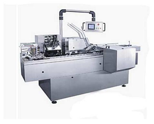
PEW-I-ZH100 Automatic Cartoning machine applies to the encase packing of blisters, vials, cosmetics, poker and similar stuff. This machine can fold leaflet, open carton and insert stuff with leaflet into cartons, printing batch number and close carton automatically.
