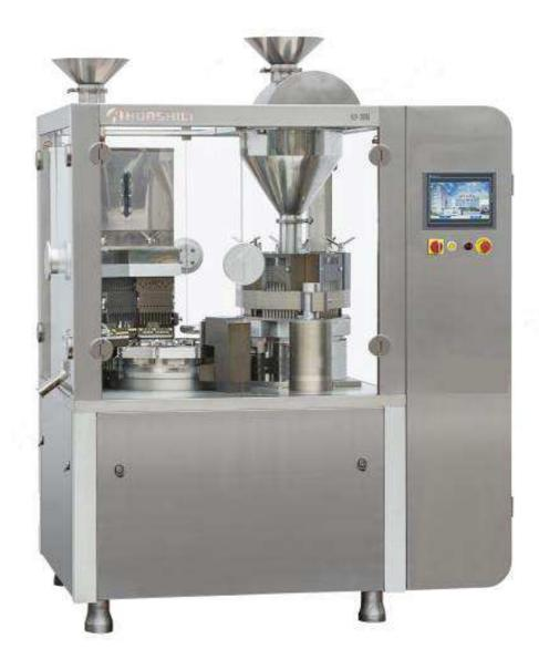
This machine is fully automatic capsule filling machines. It is suitable for capsule size from 00#-5# and safety capsule A-B
