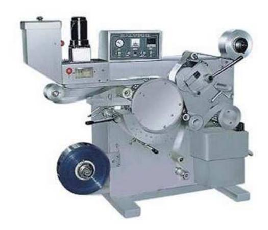
It is a small-sized Al-plastic Blister Packaging Machine designed on the base of original rolling 140 model packing machine. It is ideal equipment for small-sized pharmaceutical factory, dosage room of hospital, researching institute of medicine factory.
