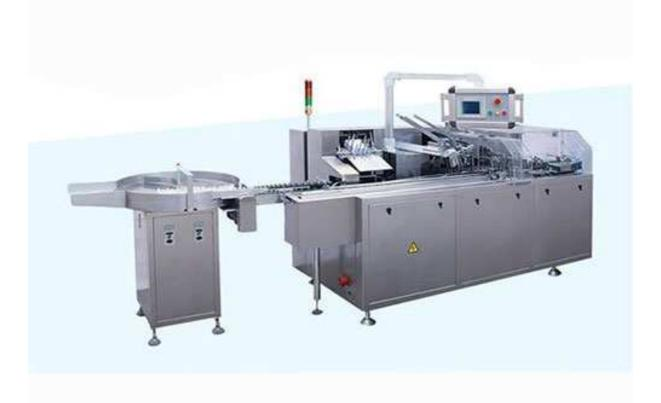
The machine is suitable for packing different sizes and specifics of tubes or similar objects with automatic leaflet folding inserting, carton opening, object cartoning, batch number embossing and cartooning sealing (hot glue sealing is an optional for the machine). It adopts PLC control with touch screen operation with all working stations equipped electronic sensor for running status monitoring.
