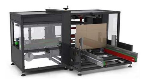
The BEM300XL Automatic Case Former is an automatic carton forming machine from Spanish manufacturer Ear-Flap. The BEM300XL Automatic Case Former has manual size adjustment, PLC control and is capable of forming up to 8 cartons per minute.
