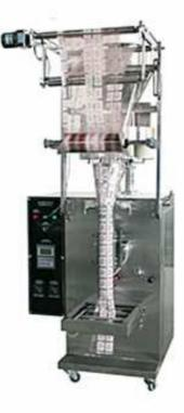
The machine is suitable for packing non sticky, bulk or granular material, such as medical pills, tea, food Stuffs, plant seeds, washing powder, coffee, sugar, desiccant etc The integrated processes of bag making, measuring filling, sealing cutting, counting and hot pressing codes can be done automatically. Packing material includes several kinds of heat seal lamination, such as PET/plated AL/PE, PET/PE, PAPER/PE, NYLON etc.
