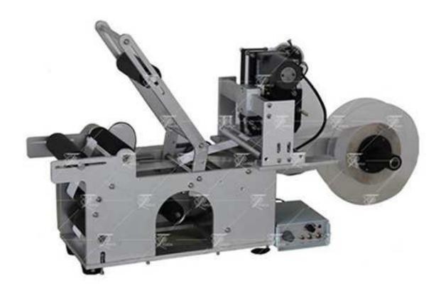
Automatic sticker machine, vial labeling machine, bottle labeling machine widely used for different sizes of round products such as round bottles, cans, jars, cylinder in daily chemicals, food, beverages, medicine and other industries
